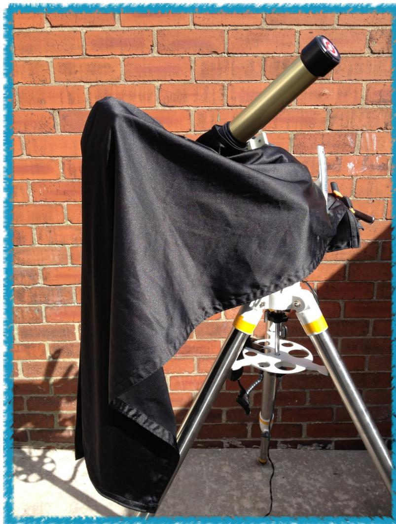
and wrap as much as possible around the camera area and this gives you a higher contrast view without any sunlight creeping in, this really does help especially on wispy prominences and filaments.
