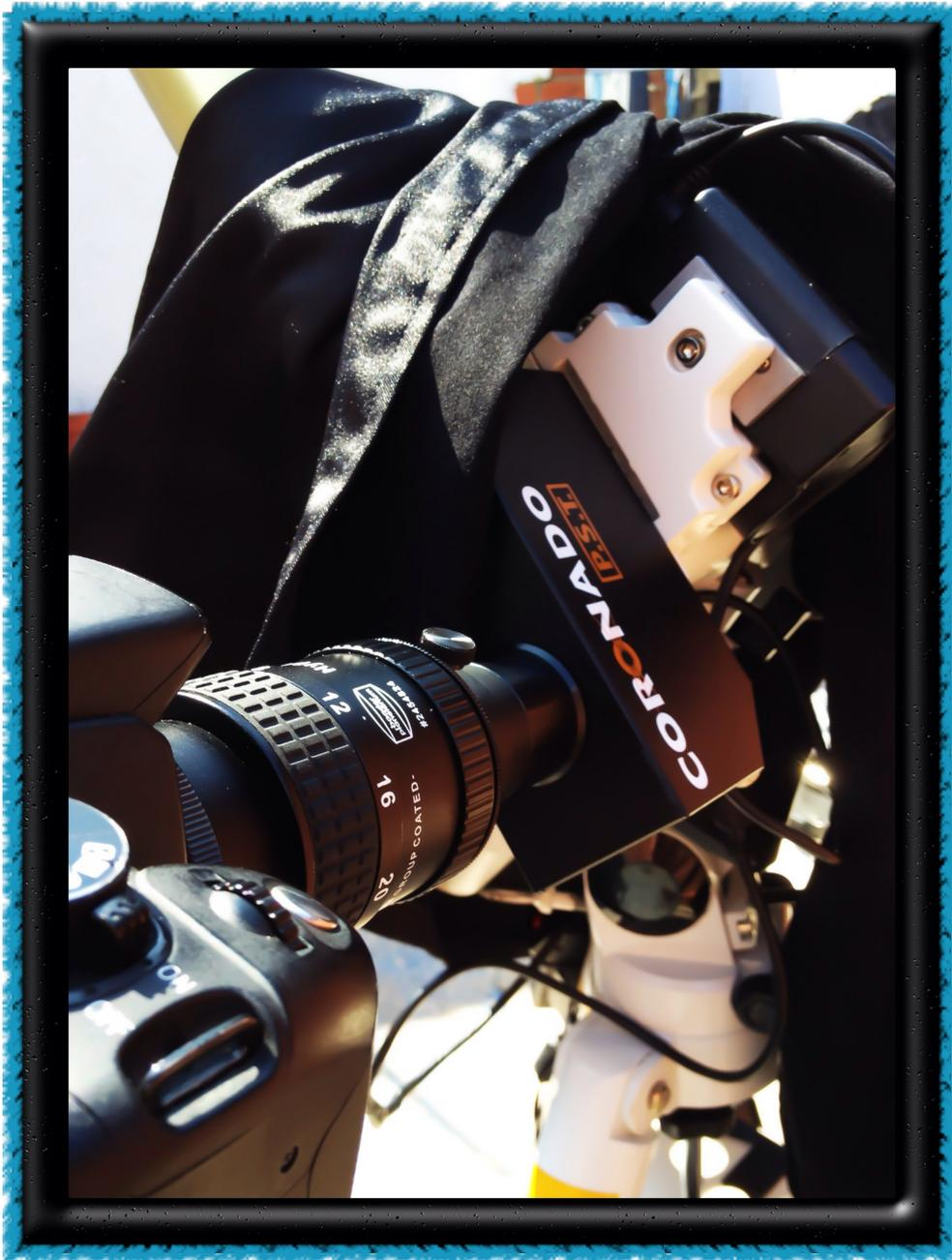
The Camera, any DSLR shooting in Raw mode and with the histogram showing, you can work out the right settings, I have found ISO200 gives best results and exposure times from 1/60th to 1/4 for prominences and 1/60th - 1/300th for disk detail. Shooting early in the morning seems best for me, as once the day and surroundings warm up, the images tend to degrade, the later in the day the worse my images tend to be.
